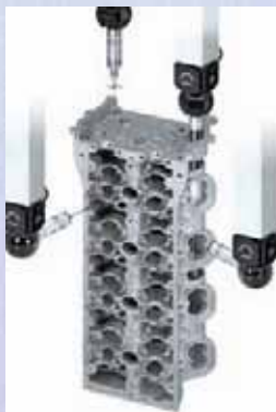
Centering point measurement
