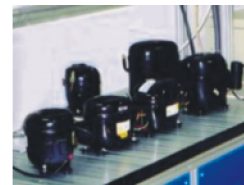
Compressor for Air Conditioner
