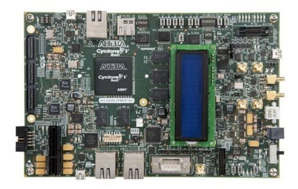
The Altera® Cyclone® V SoC Development Kit offers a quick and simple approach to develop custom ARM® processor-based SOC designs accompanied by Altera's low-power, low-cost Cyclone V FPGA fabric. This kit supports a wide range of functions, such as:
