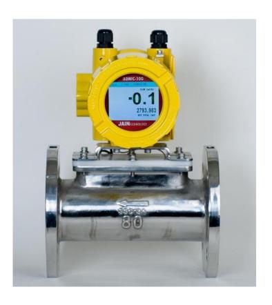
As Xonic-10G Ultrasonic Flowmeter uses Ultrasonic Transit-Time Technology, it shows superior performance than the existing pressure gas flow meter. Depends on pipe diameter size, it uses one path or three path ultrasonic sensor(s), and the temperature sensor is embedded to give compensation volume.
