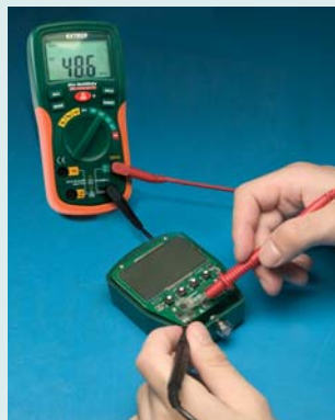
AC/DC Voltage measurements
