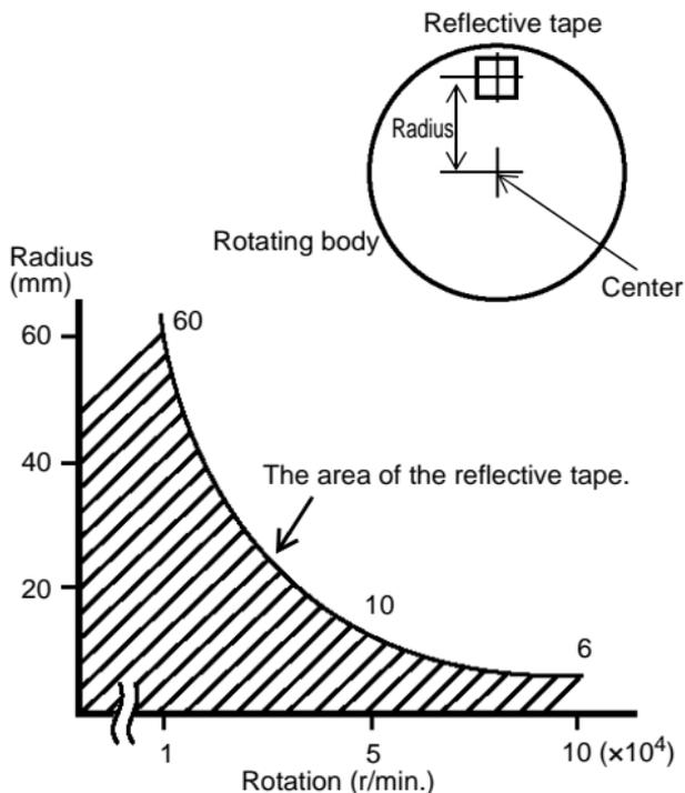
If the reflective tape cannot be attached within this detection range, increase the area of the reflective tape so that the generated pulse is 0.2 ms or higher.
