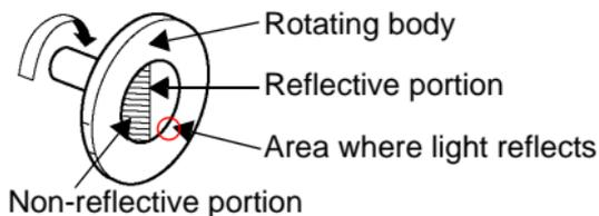
**NOTE** The red light from the instrument should be adjusted slightly off center as shown, not to the center of the rotating body.
