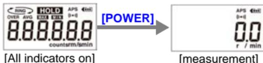
2. To turn off the instrument, press and hold the **[POWER]** key for at least 1 second.
