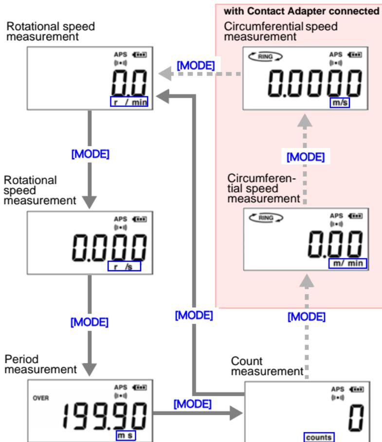
**NOTE** When selecting circumferential speed measurement, attach the 9212 Peripheral Ring to the Z5003 Contact Adapter.
