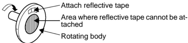
For measurement of 30,000 r/min. or higher, use the following method:
