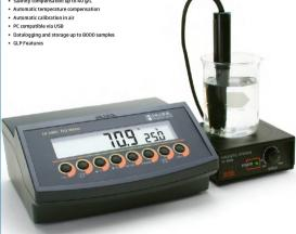
HI 2400 is a dissolved oxygen benchtop meter with automatic calibration and % or mg/L (ppm) measurement range. The measurement is automatically compensated for altitude and salinity compensation based on the user settings for altitude up to 4000 m and 40 g/L for salinity.
