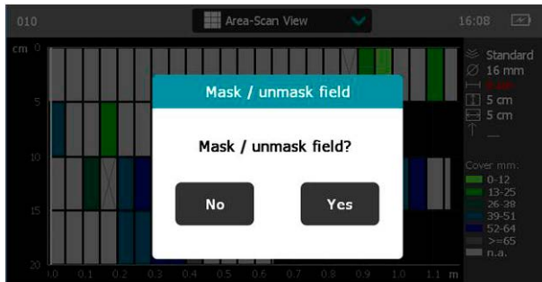
Figure 14: Area-Scan option to mask a field by double-tapping on it
