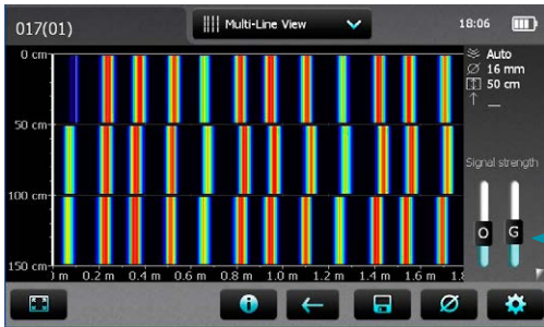
Figure 24: Multi-Line View with Signal Strength color spectrum
