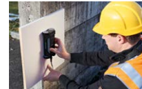
Figure 35: Scanning near to the edge
