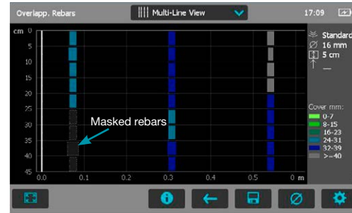
Figure 22: Multi-Line View with masked rebars
