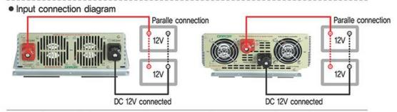
■ Input(Battery) / Equipment(Output power) Connection (DC24V)
