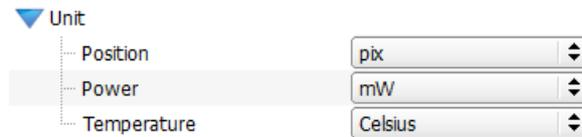
The measurement units that are displayed in the Beam Software can be selected in the **Unit** topic.
