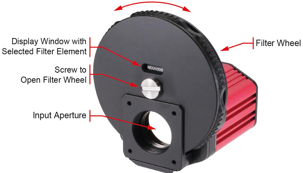
The filters come in a fixed configuration. A small window on the housing above the input aperture shows which filter is selected. The filter types and their nominal losses are model dependent as they are optimized for the wavelength of the BC207 Series model. Please find information on the pre-configured filters and links to the respective website in the tables below.
