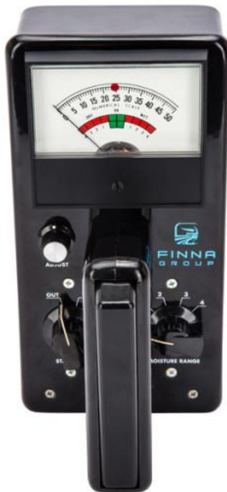
The Model N8 is designed for flat, curved, smooth, or rough surfaces such as cones or beams of yarn, rolls or stacks of cloth, rolls or stacks of paper or paperboard, carpets, tiles, etc. The electrode covers an area of 1-1/4 x 3 inches and penetrates 1/2 inch into the product. Complete with Rechargeable Battery, Carrying Case and Operating Instructions Book.
