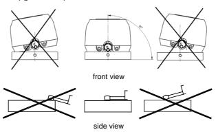
The sensor movement must be vertical to the tested surface (figure below)
