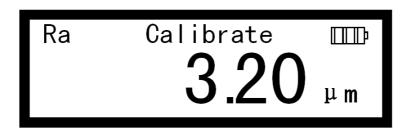
Press the Up Key and Down Key to adjust the displaying value to the value3.14.
