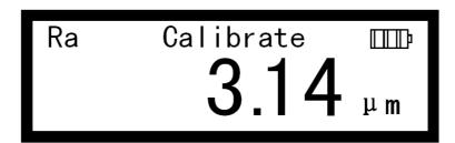
Put the instrument in the scribed line area. Sensor taxiing direction perpendicular to the scribed line of texture direction. Press the Start Key to exit the status of Calibration. Repeated many times calibration could evidently improve precision.
