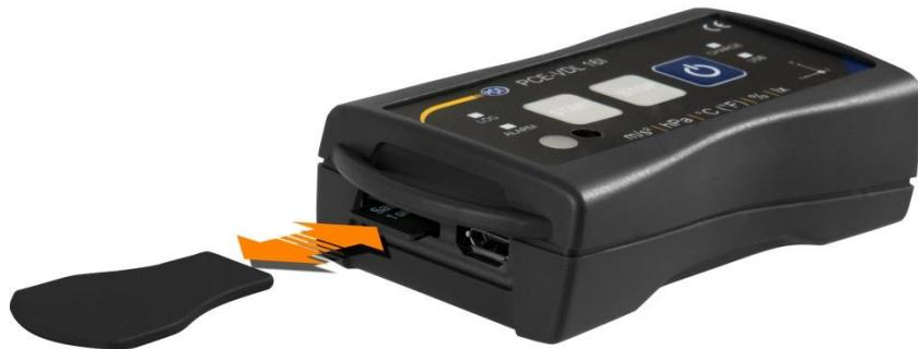
To remove the microSD card from the data logger, insert the ejector tool into the SD card slot. The memory card is then released from its retainer and snaps out of the case so that it can be taken out.
