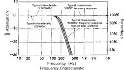
Recently there has been increased use of power through inverters, switching regulators, etc. When the high frequency noise from such appliances leaks or flows into the ground through capacitors not filtering completely, the earth leakage breaker may trip even though there is no "actual" leakage. In such a case, the instrument do not give leakage current reading if "50/60Hz" frequency response is
