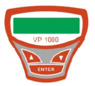
• Switch the Viscometer on by pressing the "ENTER"-button for 6 to 10 seconds. The following read out appears on the display with the battery symbol.
