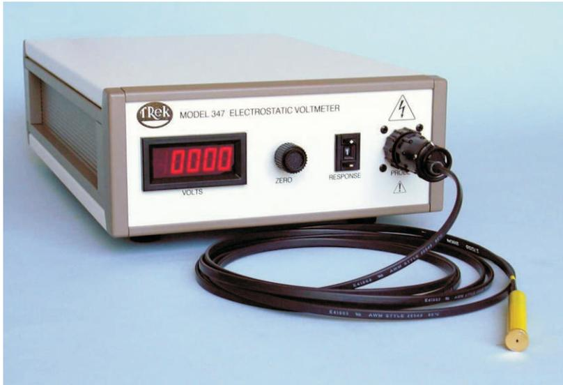
The Trek Model 347 is a precision electrostatic voltmeter for making noncontacting surface voltage measurements in the range of 0 to  $\pm 3$  kV DC or peak AC.
