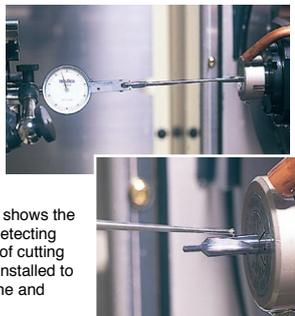
The photo shows the scene of detecting deflection of cutting tool edge installed to the machine and deflection.
