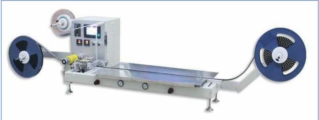
Tape & Reel Packing: Automatic seal, scroll and manual place the component.
