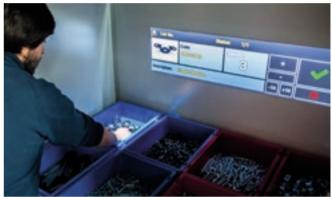
**IRIDE™, the innovative interactive control system\*** makes storage and retrieval faster, more accurate and more intuitive using a digital environment, fully-integrated with both the storage system itself and our management software, ICON™ and has 4 main functions:
