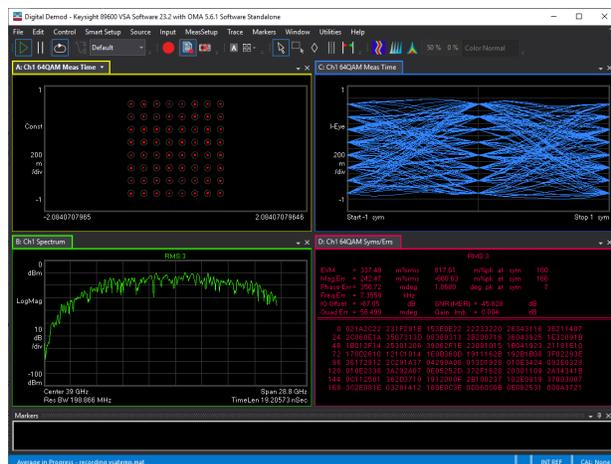
Figure 4. QAM-64, 16 GBaud at 39 GHz carrier
