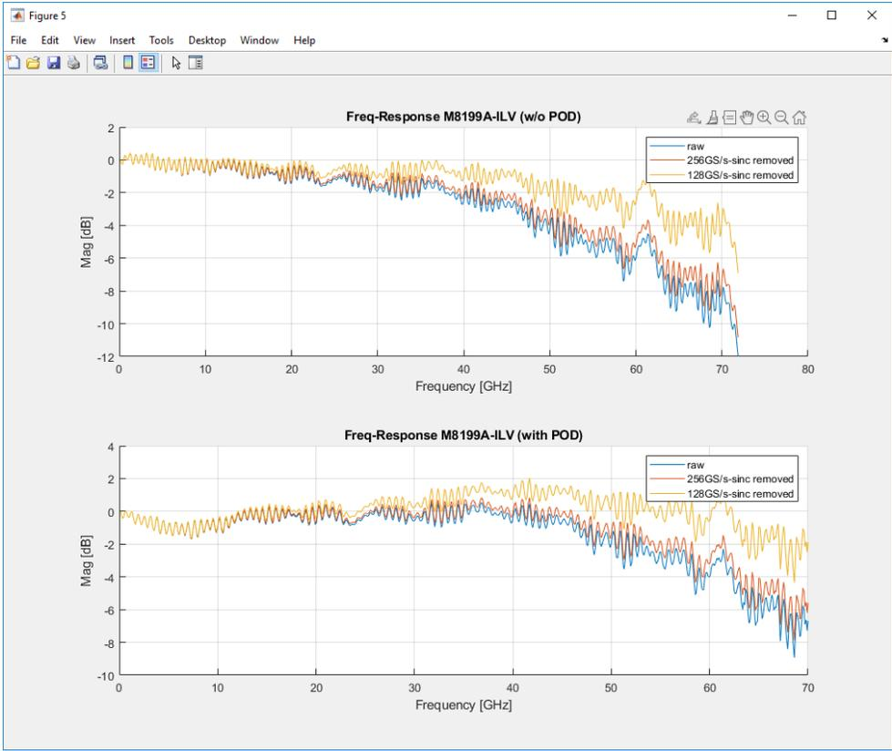
Figure 6. Frequency response M8199A with Option ILV (top), and options ILV+ remote-remote head (bottom)
