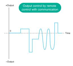
AC opration range (with 50 Hz or more frequency, 50% of duty cycle and without any DC bias)
