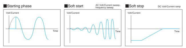
Applications: Power activation test, various start-up tests of motor, etc. fluctuation test of wave shape and so on.
