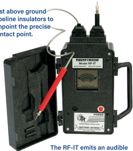
The RF-IT emits an audible beep. When the operator gets closer to the point of contact the unit starts beeping faster. At the same time, the LCD meter moves from left to right.
